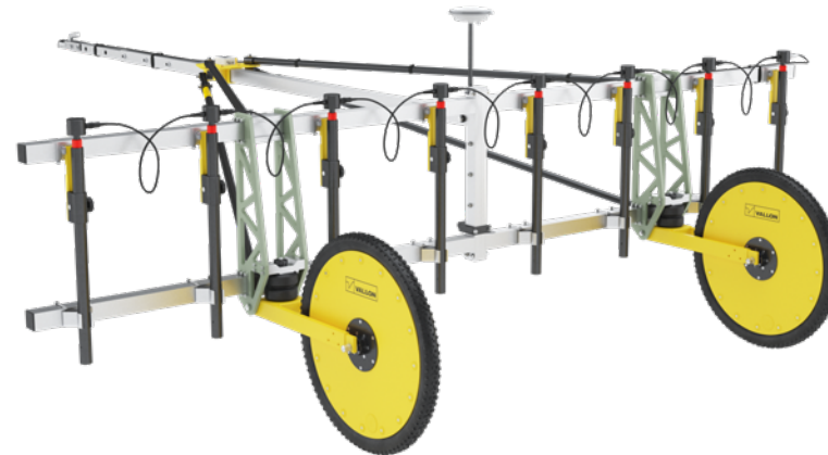
Trailer VXVT wide – Prepared for up to 8 probes with a distance of 50 cm (shown with optional components)
